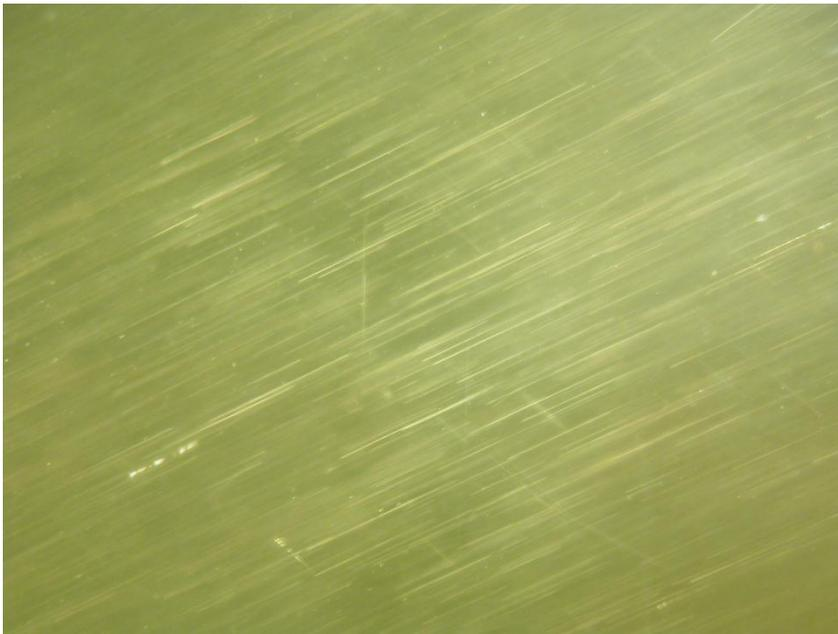
*Figure 5: One of the sets of needles was arranged only in one direction and was much denser; this gave rise the stronger ray as seen in figure 2. Photomicrograph by M.B. Vyas, magnified 60x*
