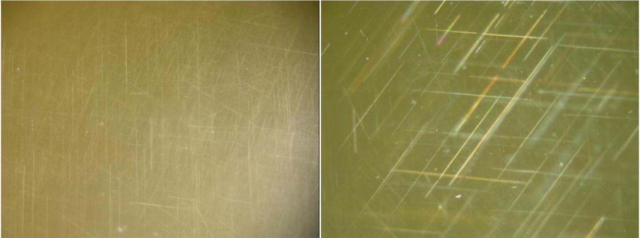
*Figure 6: Two different sets of intersecting needles were observed. One set comprised two-directional needles which intersected each other at an angle of nearly  $90^\circ$  (left) while in another set the needles appeared to be intersecting at approximately  $60/120^\circ$  (right). Also note the iridescent and brownish appearance of these needles. Photomicrographs by M.B. Vyas (left) and G. Choudhary (right); magnified (left) 60x and (right) 80x*
