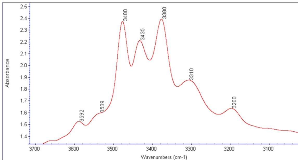
Figure 8: Infrared spectrum of this multiphenomenal quartz in the region  $3000 - 3700 \text{ cm}^{-1}$  shows peaks that are consistent with natural quartz
